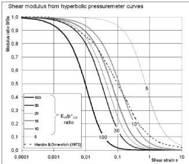
Figure 6. Typical  $G/G_0$  versus  $e$  graphs for various soils from the extrapolation of the pressuremeter hyperbolic law.
