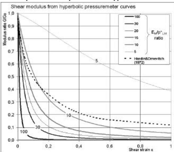
Figure 7. Graphs of  $G/G_0$  versus  $e$  in arithmetical scale.
