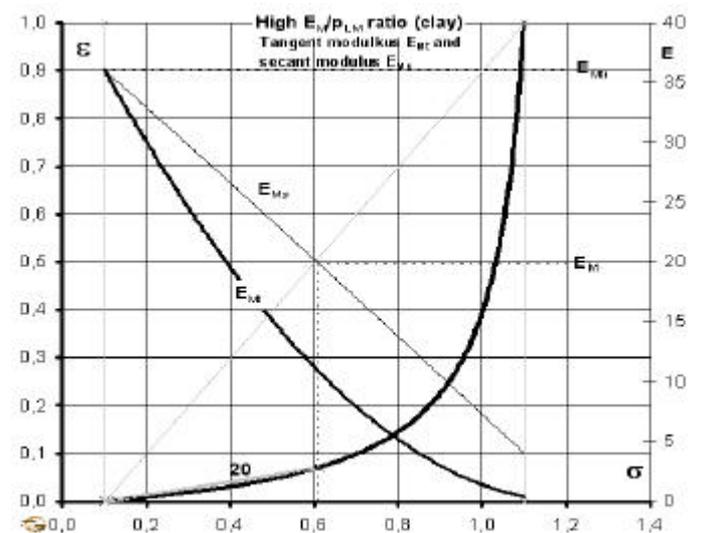
Figure 5: Example of the secant and tangent E-moduli  $E_{Ms}$  &  $E_{Mt}$  versus the stress level  $s$  (typical hyperbolic MPM curves in sandy or clayey soils).
