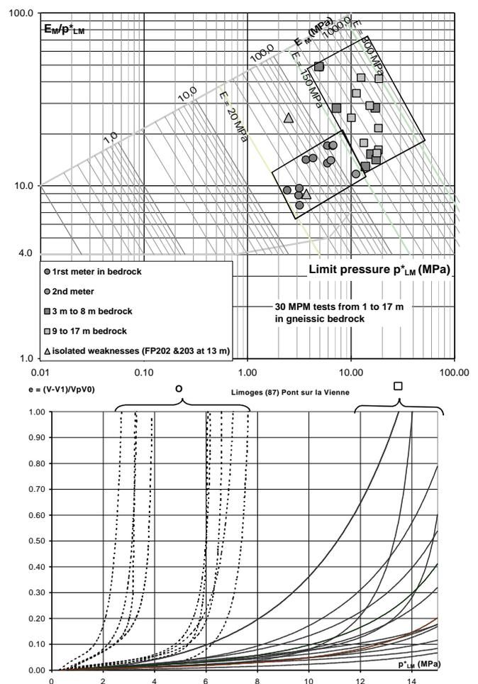
Figure 1 – Pressuremeter tests in weathered gneiss
