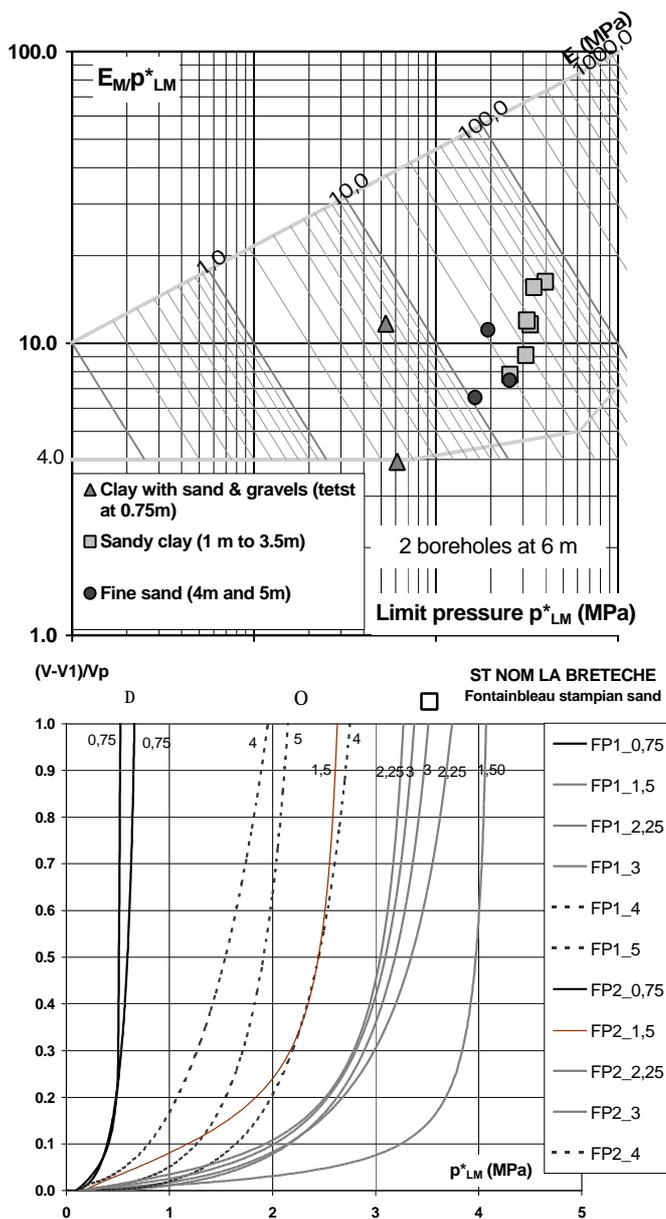
Figure 2 Pressuremeter tests in sand
