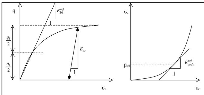
Figure 4. Schematic response for tri-axial and oedometer tests by Plaxis-HSM.
