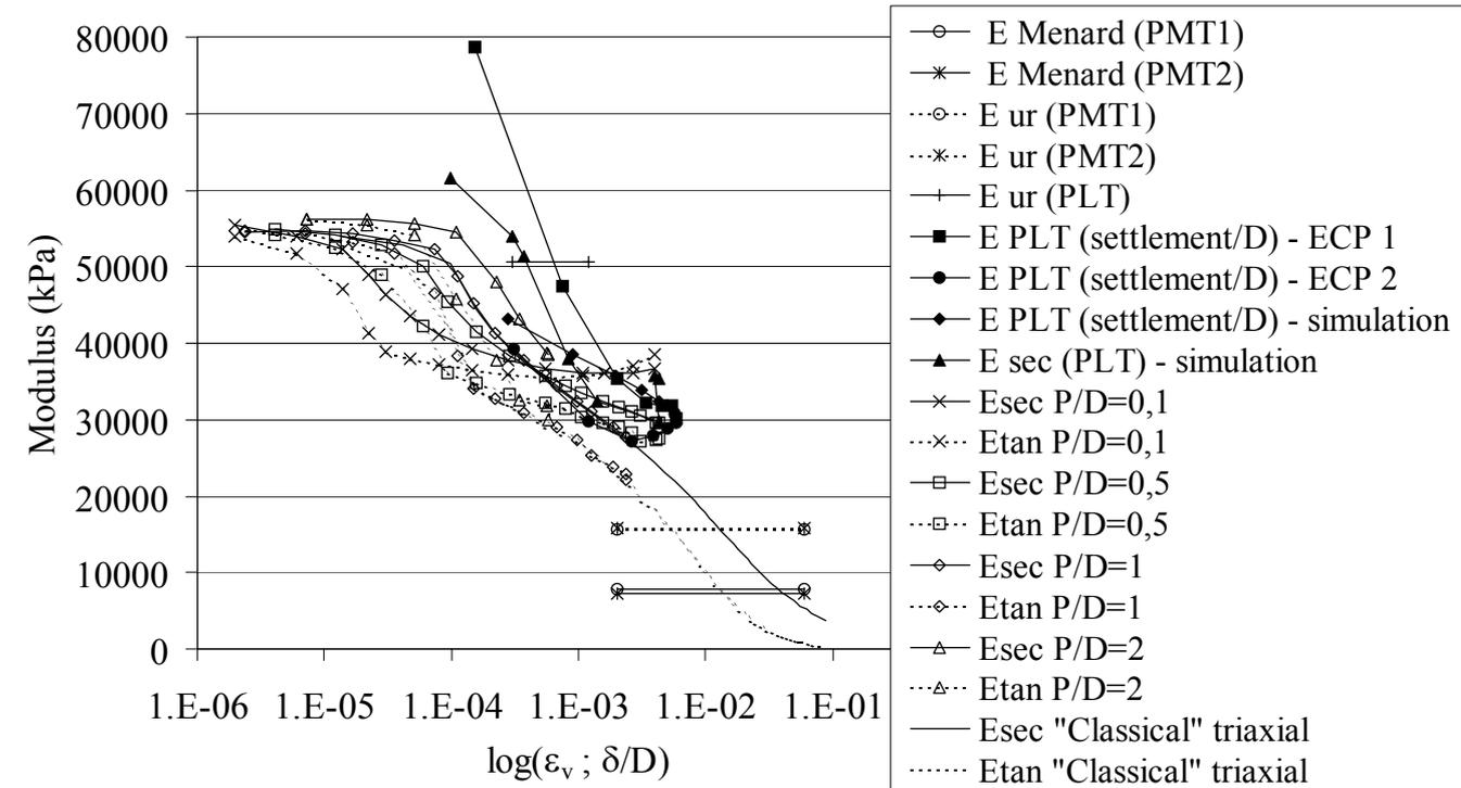
Figure 11. Moduli as a function of strain level for various numerical simulations and test analysis.
