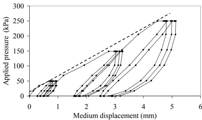
Figure 7. Plate load test results according to ASTM-D1196 standard.
