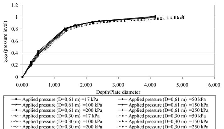
Figure 8: Ratio of the settlement at a given depth and the total settlement ( $\delta/\delta_s$ ) as a function of the ratio between this depth and the diameter of the plate ( $z/D$ ).
