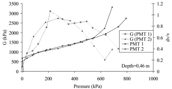
Figure 3. Proposal for obtaining tangent shear modulus  $G$  in the pseudo-elastic zone.
