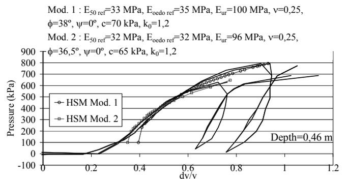
Figure 5. Best fitting curves of two pressuremeter tests using Plaxis-HSM.
