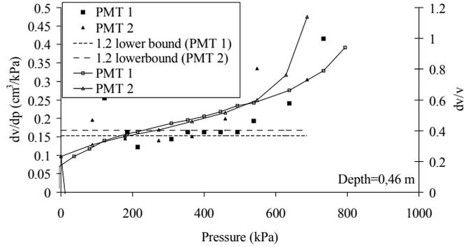
Figure 2. Definition of the pseudo-elastic zone for tests PMT1 and PMT2.
