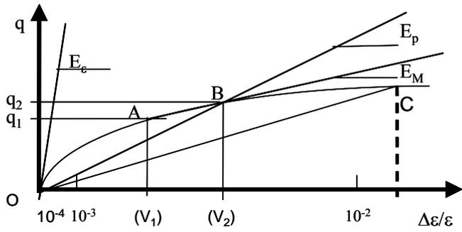
Figure 1. A typical stress-strain curve example showing tangent and secant moduli.
