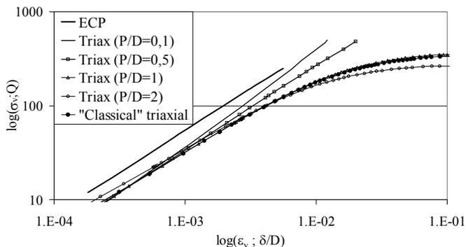
Figure 12. Comparison between tri-axial test strain and PLT strain
