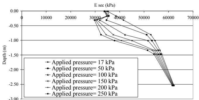
Figure 9. Variation of the secant modulus with the depth.
