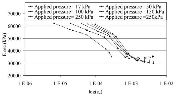
Figure 10. Variation of the secant modulus with strain.
