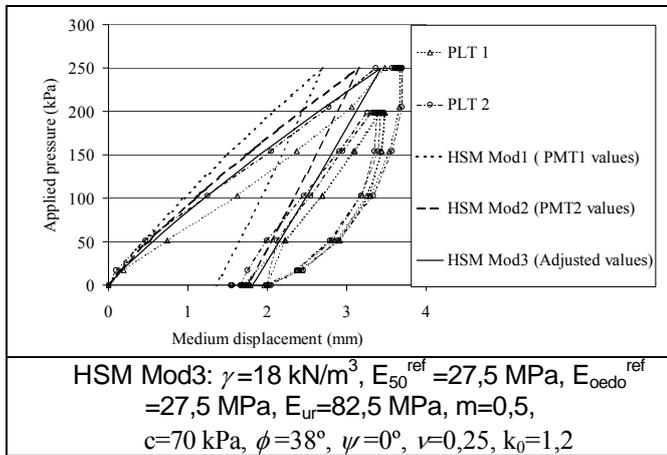
Figure 6. Plate load test results according to LCPC-CT2 procedure and best fitting curves.
